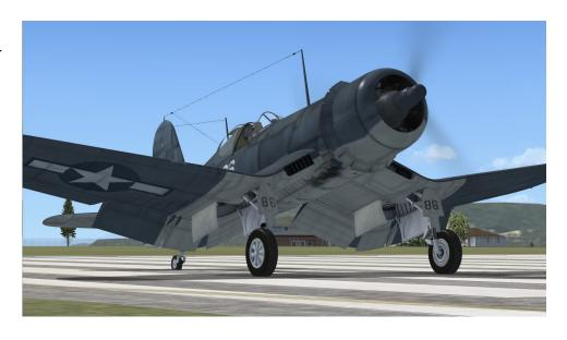
was specified. This resulted in removal of the two 30 caliber nose guns and the addition of a single 50 caliber in each wing for a grand total of four. The additional guns required elimination of the wing fuel tanks and to regain that lost fuel capacity the fuselage was lengthened by 18 inches to provide room for a center fuel tank. Unfortunately this meant the cockpit had to be moved back by 3 feet, further reducing the pilot's forward visibility.
